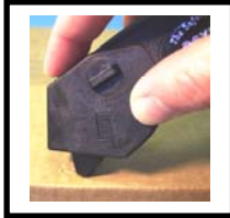
Sprung release lever is pushed forward to unlock guards
