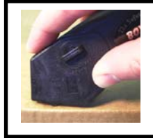
With lever forward pierce into box
