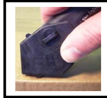
Remove thumb/finger from release lever when cutting
